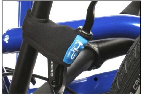
fig. 1 Mounted brake lever cover
