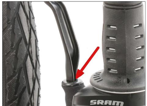
fig. 2 The arrow shows where to put some silicone on
