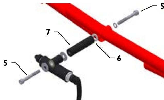
With the Tandem Coupling you can transform two trikes into a trike tandem. Just mount the coupling to the towering trike, remove the front wheel of the second trike and attach the fork dropouts to the coupling. The tandem coupling is only suitable for operation on non-motorized trikes.
